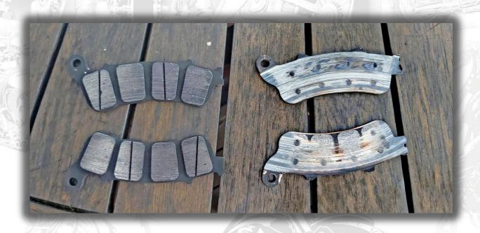
Honda Fury brake pads. Rear brake pads have been worn down to bare metal — Luckily enough for Hippy the fault was found and pads were replaced without any incidents on the road.
