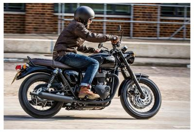
There are also two engine modes – Road and Rain – available through a control on the right switchblock which softens throttle response for wet roads. Unlike most of these, it doesn't make the bike feel dead and detached, just more controllable.
