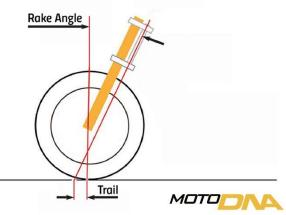
is always self-centering as a torque is generated at the tyre contact patch keeping the wheel straight.
