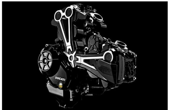
For the very first time on a Ducati, transmission is of the belt type. To mount the front pulley the engine cover has been specially redesigned. The final 28/80 ratio corresponds to a drive ratio of 15/43. The XDiavel exhaust is a 2-in-1 system
