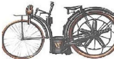
The interesting feature of this **1892 five cylinder Millet** from France was the five cylinder rotary engine in the rear wheel. The cylinders and the wheel turned while the crank was stationary. This was not the last time that such an engine was used in a motorcycle, although the next one to use this design had the engine mounted in the front wheel.
