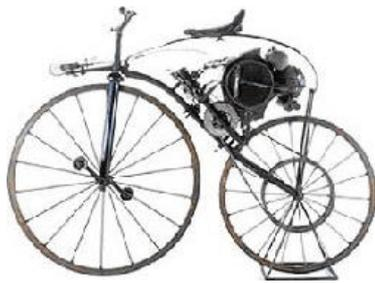
This— **Michaux-Perreaux Steam Velocipede**— built in 1868-69 in Germany is an elegant machine. Built on the **Michaux** “boneshaker” bicycle, the frame was modified and seat raised to allow room for the **Perraux** steam engine. Pulleys and drive belts were added to power the rear wheel. This machine kept the front pedals.
